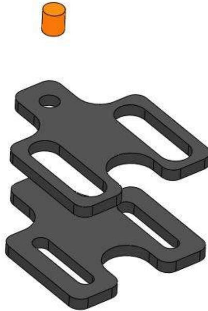
1. Apply acrylic solvent (which we all refer to as acrylic glue) liberally to the Slider bottom.
