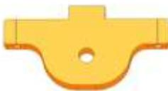
Use the drill press. Place part in vice with tab facing up. Place the part 4.3 such that the slot fits on the Pivot Plate tab. Use the part 4.3 clearance holes to align the 4-40 tap holes for the Pivot Plate.
