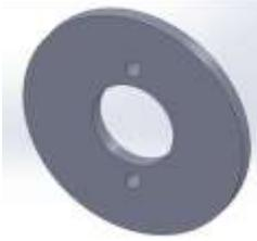
**Countersink** with an 82° countersink suitable for 4-40 flathead screws. Screw does not have to be flush when placed in. Err on the side of being slightly under countersunk.
