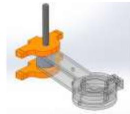
5. Using 4-40 screws with lock washers (see TA robot) install pivoting assembly onto the mounting fixture as shown below.
