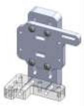
1. Put together assembly using 8-32 fasteners as shown to the left. (Also see TA robot)
